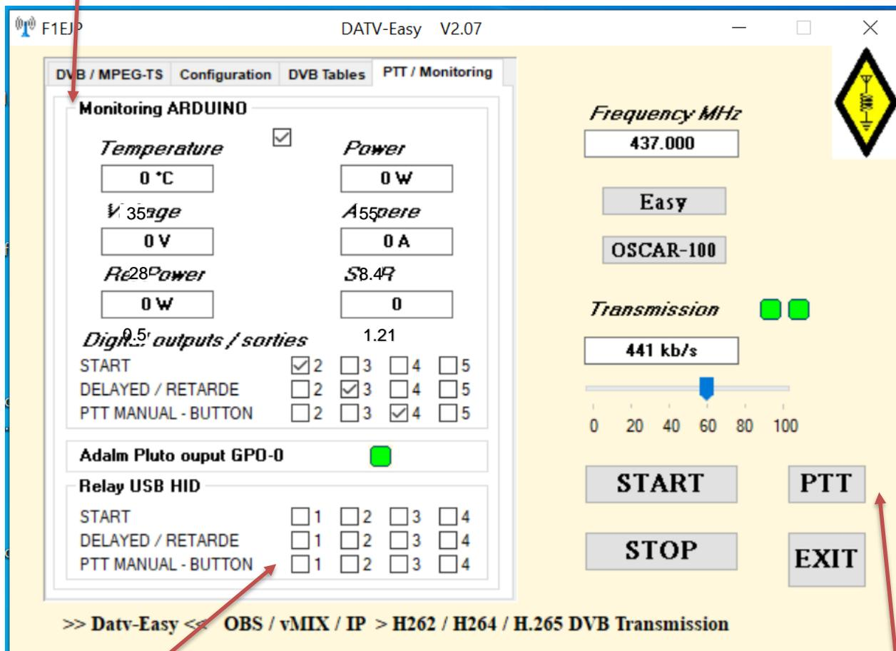
To control the power supplies of your amps without or with delay or manual to avoid calibration peaks :
