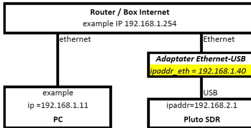
The PlutoSDR once connected as in the diagram, should automatically have an IP address given by your network router (router, internet box).
