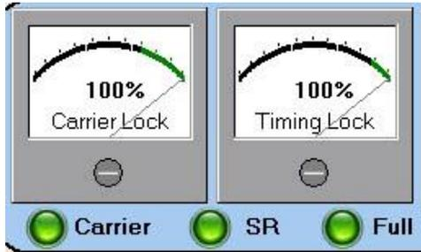
The first thing to do to acquire a TS in Tutioune: Having the 2 first LED going green. Timing(SR) and Carrier PLL are locked. As long as one does not have these 2 green LED, no need to look further.
